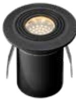
Onyx 30 RA (241D) Aluminum - Anthracite LED 0.5 W 2,700 K 1 lm 59 x 45 mm (H x Ø) Drill hole 30 mm
